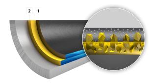
ILAFLON Resist R Plus FF is a strongly ceramic reinforced system with excellent performance in abrasion resistance, durability of non-stick effect and cleanagility. For top level baking and roasting applications
