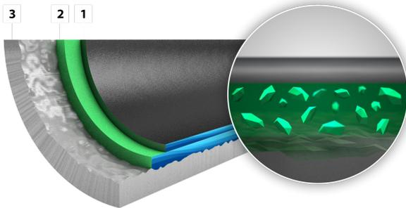
CERALON is an one-coat or a two-coat system with high hardness, which combines excellent temperature stability, good non-stick properties and outstanding cleanability. Due to a low curing temperature in production, CERALON has a lower energy consumption in comparison to standard coatings.
