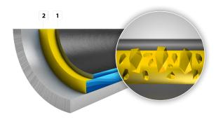
ILAFLON Resist SP-800 PFAS-free is a two-layer barrier-optimized anti-adhesion system with very good performance.
