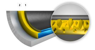
ILAFLON Resist Plus PFAS-free is a ceramicreinforced resin combination system with the best usage properties. A versatile coating for the entire range of baking, grilling and roasting tins.
