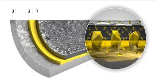
DURIT Granistone HL is an outstanding threelayer non-stick coating without ceramic reinforcement in the mid layer. DURIT Granistone HL is based on the DURIT High Level technology with a special polymer matrix. This technology guarantees a good non-stick effect and excellent abrasion resistance also in intensive use. DURIT Granistone HL set itself apart due to its high quality hard and rough surface.
