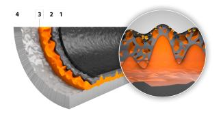
DURIT Professional P is a three-coat system based on a innovative multi-polymer combination specially developed by ILAG. This coating is unique, due to it's wavy structure. Thereby it convinces with an extremely robustness. Therefore it is possible to use metal utensils to stir foodstuff in the cookware product.
